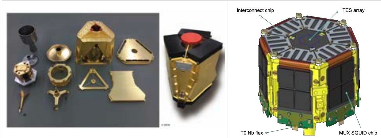
Figure 13. Left) Left: The various sub-assemblies of the FPA-DM during integration. At the top left the Niobium shield is shown. The triangle in centre is one of three Kevlar cord assemblies which, together, form the suspension of the T1 stage. The hexagonal structure on the left is the partially assembled detector stage (see right figure). On the right, the first FPA-DM completely assembled. The front-side red cap is a protective cover to avoid contamination of the optical filter. The three front black covers will be replaced by the readout harness during further tests. The black back-side cover protects the sensitive electronics and internal harness of the FPA during transport and handling (van Weers et al., 2022, SPIE, submitted and AthenaNuggets43). Right) Preliminary design concept of the T0 (50 mK) detector assembly. The TES array is mounted at the top of the structure and wire-bounded to an interconnect chip. Each carrier/interconnect chip holds 4 MUX SQUID chips with Indium bump-bonds realizing the required high-density, low-impedance contacts between the carrier and MUX SQUID chips. As a baseline, the Nb flex harness from the FPA's T2 stage will be glued to a rigid support that is mounted below the Carrier chip, allowing wire-bonding directly from the Nb flex harness to the carrier chip.
