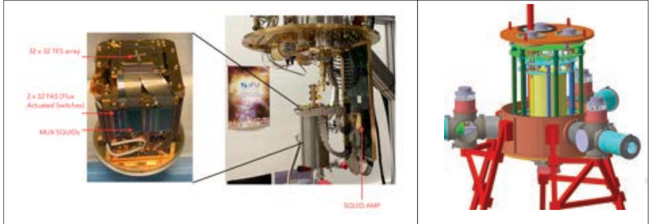
Figure 26. Left) The snout is composed of a 1024 TES array with its associated cold readout electronics. The snout is placed in the niobium shield and connected to the 50 mK stage. Superconducting looms insure the signals connection to the 500 mK terminator card and then to the 3 K cold electronics 82 (see Castellani et al., 2022, SPIE submitted). Right) Conceptual scheme of the cryostat for testing and calibrating the Focal Plane Assembly of Athena/X-IFU. Credit: INTA – C2CC team (and AthenaNuggets62).
