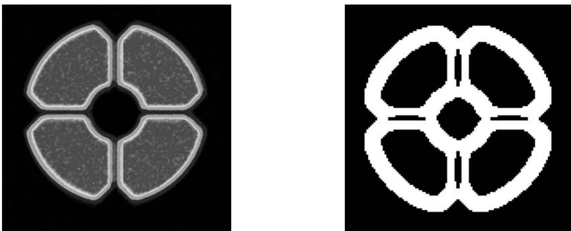
Figure 64: A simulation of OWL metapupil (left) and the mask selection for the star enlargers tip tilt calculation and nulling (right).
