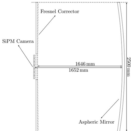
Figure 1: Sketch of the MUCH telescope optical system.
