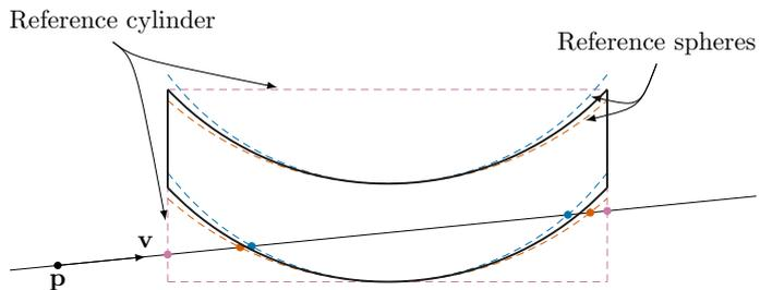
Figure 2: Example of the ray tracing through an aspherical shell. Intersection points of a ray moving in the direction  $\mathbf{v}$  from point  $\mathbf{p}$  are numerically computed using reference surfaces to constrain the root-finding interval.
