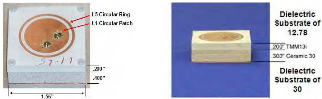
Figure 2.10: Top and Side Views of Dual-Band Co-Planar Patch Antenna.
