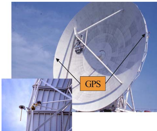
Fig. 1 Positions of the two GPS antennas installed on the VLBI telescope
