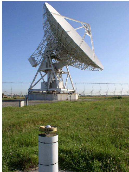
Figure 1. The Medicina (Bologna) VLBI telescope: an AZ-EL 32 m steerable antenna mount whose twin telescope is located in Noto (Siracusa). In the foreground of the picture the IGS GPS antenna co-located with the VLBI telescope is visible.
