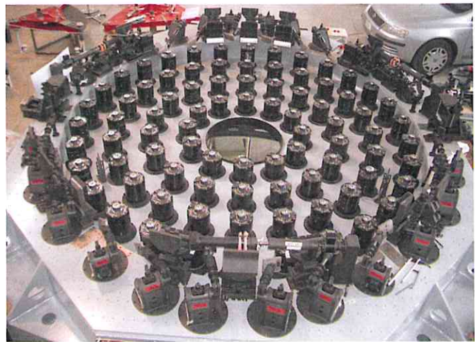
Fig. 2 – The axial and lateral supports before the installation of the mirror (top view).
