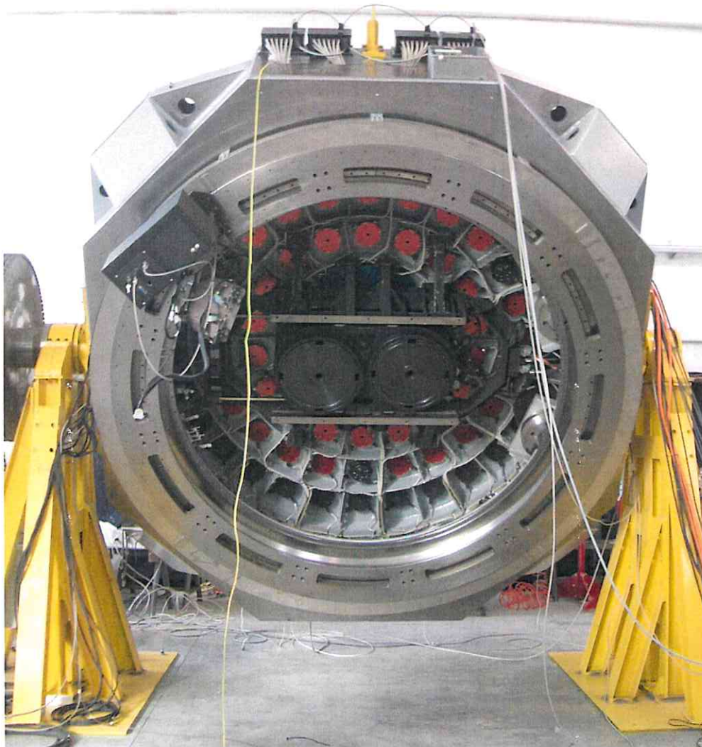
Fig. 8 – The ADC assembly mounted on the backside of the primary mirror cell. Metallic dummies are installed in place of the prisms. The telescope is equipped with two sets of refracting elements which can be exchanged: the ADC (right side in the picture) and a field corrector (left).
