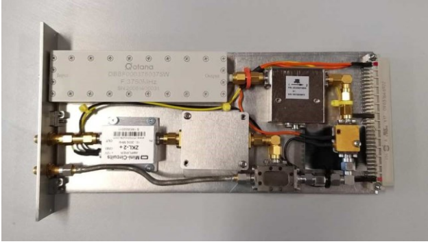
Figure 5: assembled RF down converting board
