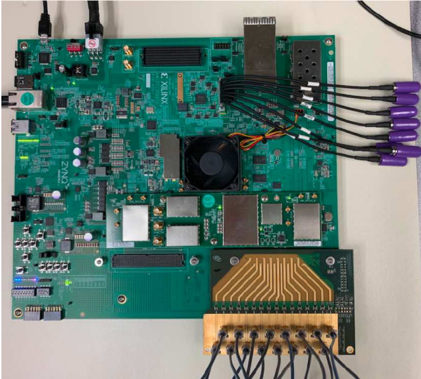
Figure 5. Picture of one Xilinx ZCU216 RFSoc evaluation kit. A mezzanine board, shown on the lower right side, will be used to connect the ZCU216 with the RF module (outputs of the signal conditioning modules).
