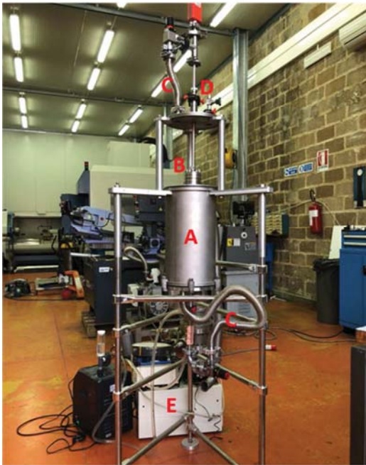
Fig. 4. Proprietary developed experimental apparatus with indication of main items: (A) vacuum chamber; (B) experimental cell; (C) vacuum circuit; (D) feed-through system for power, control and signal connections; (E) vacuum pump.
