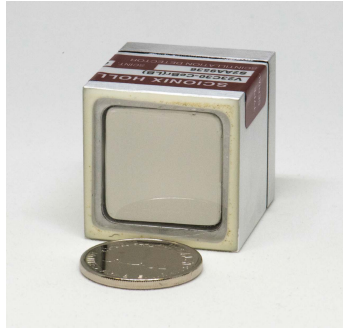
Figure 2: The 23 \times 23 \times 30 \text{ mm}^3 \text{CeBr}_3(\text{LB}) crystal by Scionix used in the present work shown next to one UAE Dirham coin.
