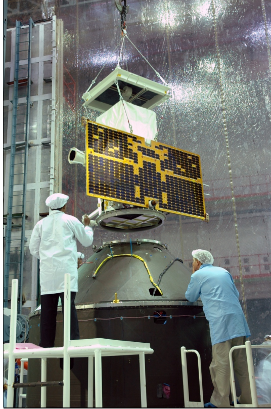
Fig. 3: The AGILE satellite during integration with the launch vehicle (Shriharikota, India, 2007).
