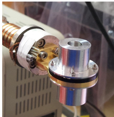
Figure 3. Filter sample mounted on the cold finger of the JASCO FT-IR 410 cryostat. The sample (black anodized aluminum frame) is thermally anchored to the gold plated copper fixture and protected by two aluminum radiation shields opened only along the beam optical path.
