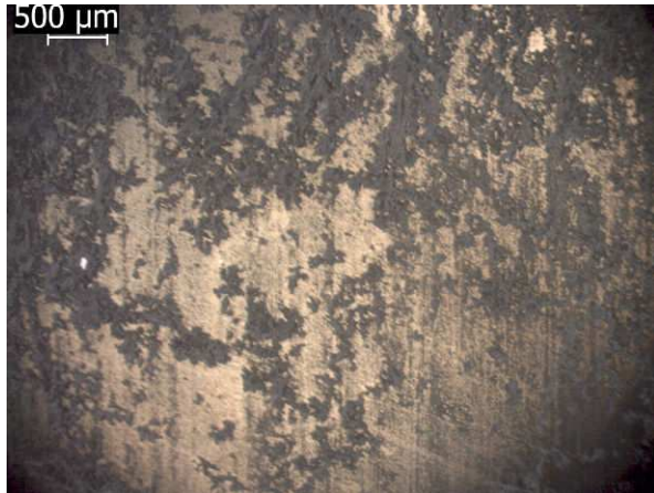
FIGURE 4. Tin plating on oxidized Cr: the chromium was not dissolved; there are traces of tin deposit on the surface.
