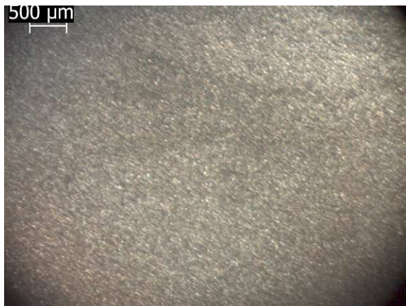
FIGURE 5. Tin plating on Ge + SOG + Cr + Cu treated with hydrogen peroxide: the deposit is uniform and defect free.
