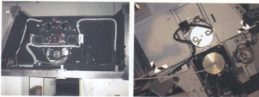
Fig. 2.2 – The OIG filter wheel inside the Nasmyth-A instrument adapter (left side). OIG and ARNICA in operation at the telescope (right side).
