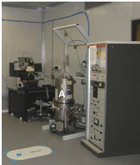
Figure 4 – Evaporation beam equipment in the INAF-OAPA XACT facility clean-room.
