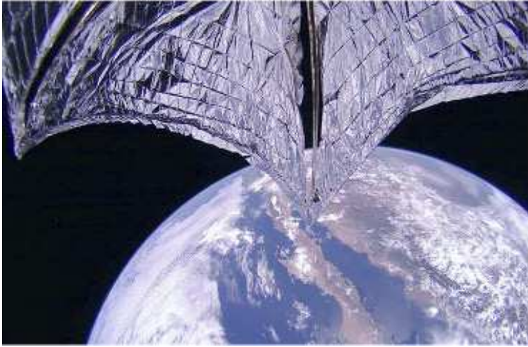
Fig. 8 An image taken on 25th July 2019 showing the successful deployment of the Light-Sail2 solar sail. (Image credit Planetary Society)
