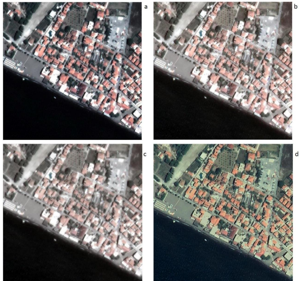
Figure 2. The image of the same region in Figure 1, after being processed by pan-sharpening techniques: (a) multiplicative method, (b) simple mean method, (c) IHS, and (d) Brovey transformation.
