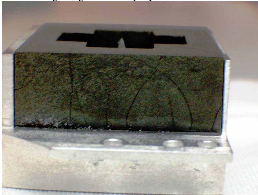
Figure 2: Lateral view of the damaged target
