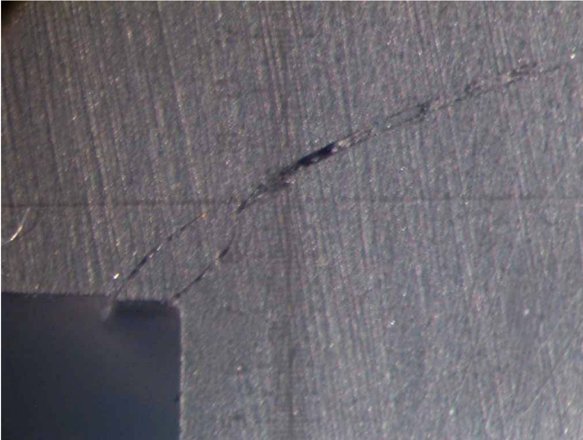
Figure 7: Details View through a microscope of the crack on the 44 GHz target (id parte)
