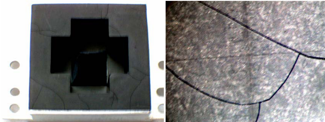
Fig. 45 Cracks on the lateral 30 GHz target (left) and detailed microscope view (right)
