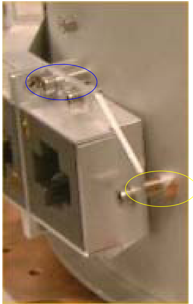
Fig. 5 The sample is mounted on the shield by means of six stainless steel screws and washers (blue line). The lateral fixation is fitted to the cylindrical wall by means of copper adaptors (yellow line).
