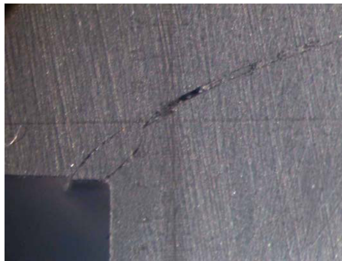
Fig. 46 Microscope image of the 44 GHz crack
