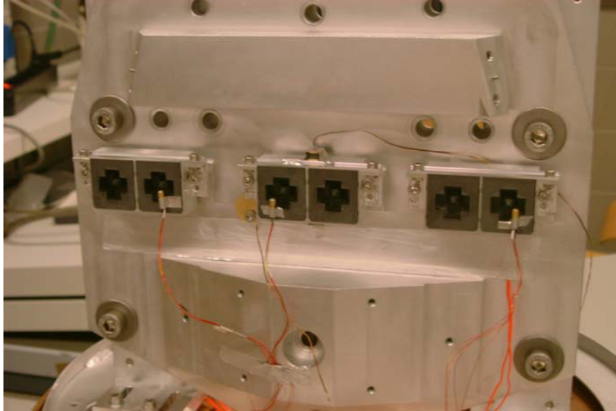
Fig. 9 The samples are mounted on the fixture by means of two stainless steel screws and washers. Temperature sensors are visible.
