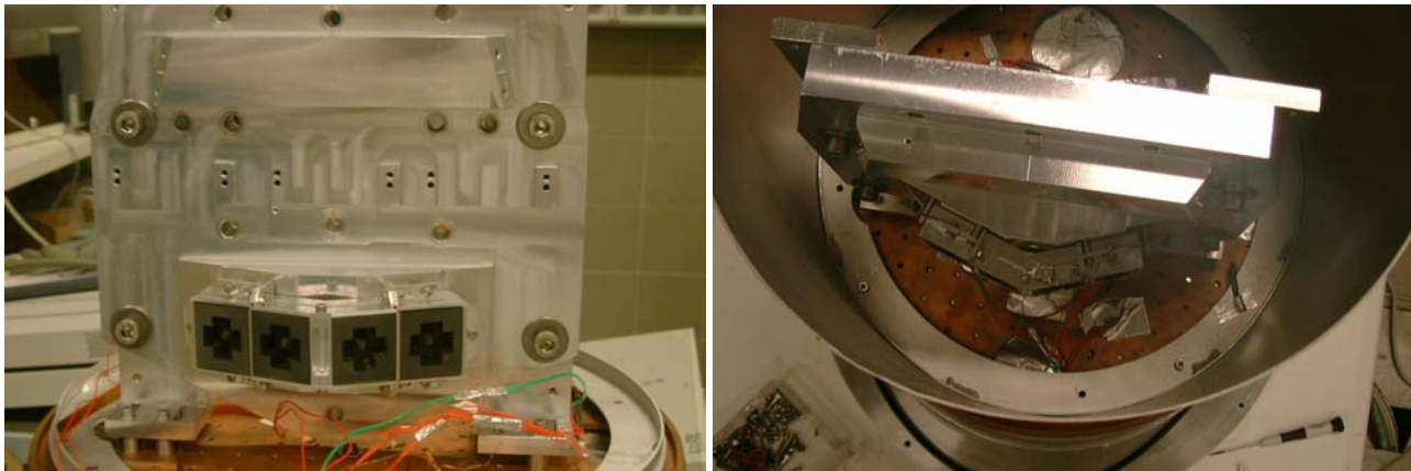
Fig. 1 The 30 GHz Reference Load mounted on a dedicated structure, whose interfaces are representative of the HFI 4 K shield ones (left), surrounded by a radiative shield, representative of the LFI main frame environment (right, top view).
