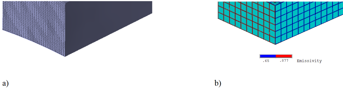
Figure 6 –MM simplified model. Each Si stack is composed by thousands of pores (a). The Finite Element Model is composed by much less solid elements (b). The emissivity of the pores side is different from the other Silicon surfaces.
