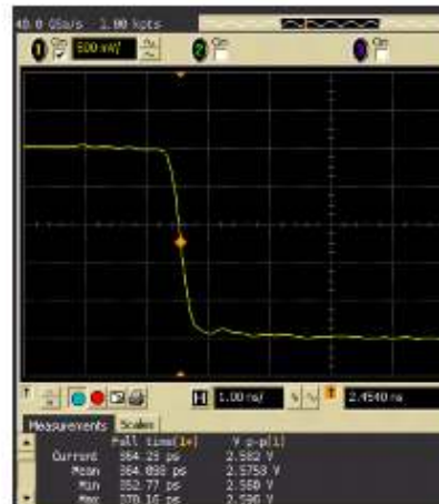
Fig 1b: Example fall time of 364 ps
