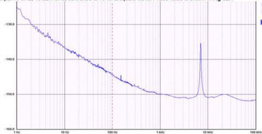
Fig 3a: Phase noise of 10 MHz square wave output, input 10 MHz sine input 13 dBm to input A.
