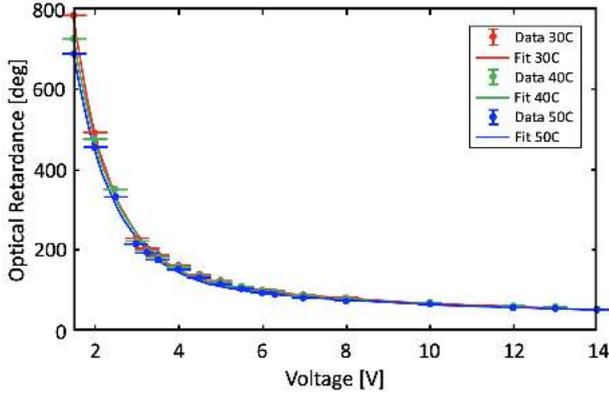
**Fig. 3.** Optical retardances for different applied voltages and verification of the PMP performance for different temperatures (Casti et al. 2018).
