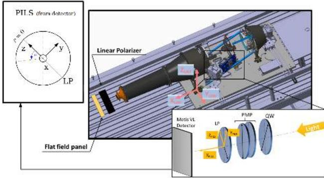
**Fig. 4.** Schematic view of the set up used for data acquisition and Metis polarimeter optical elements relative orientations in PILS reference frame [compared with the Unit Reference Frame (URF)]. The arrows in the optical elements represent, respectively: the fast axes for both the QW and the LP, and the PMP polarization axis.
