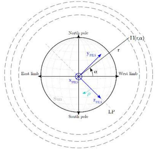
**Fig. 5.** Positions of the sensor's elements,  $H(r, \alpha)$ , for the LCVR retardances evaluation in Eq. (5). We considered different heliocentric distances,  $r$ , from  $3.14 R_{\odot}$  to  $3.63 R_{\odot}$  and different polar angles,  $\alpha$ . The PILS reference frame position relative to the Sun is shown in blue. In particular, the  $z_{\text{PILS}}$  axis results were found to be at  $-45\text{deg}$  from the west solar limb.
