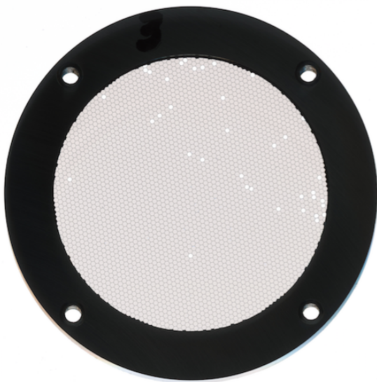
Fig. 53 – Scanner image in transmission mode of the sample filter M3 and M4 at the end of the S5/R5 level vibration tests.
