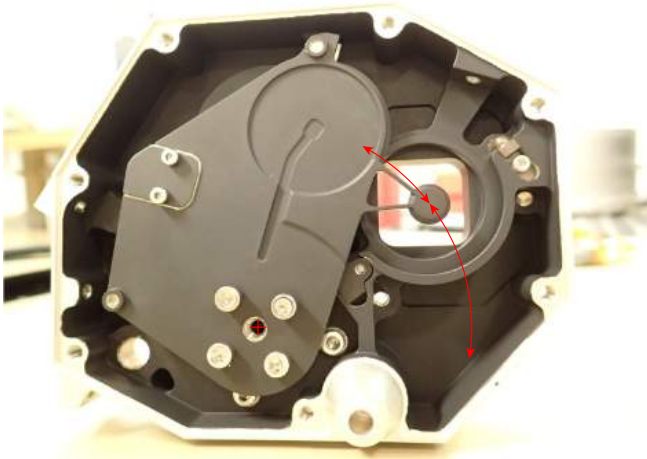
Fig. 4. Entrance door of FSI, looking towards the Sun. The occulting disk is held off the door lid by two supporting rods. The occulting disk is shown in position. Rotating the lid around its axis (red cross) clockwise closes the door, rotating it counter-clockwise opens it.
