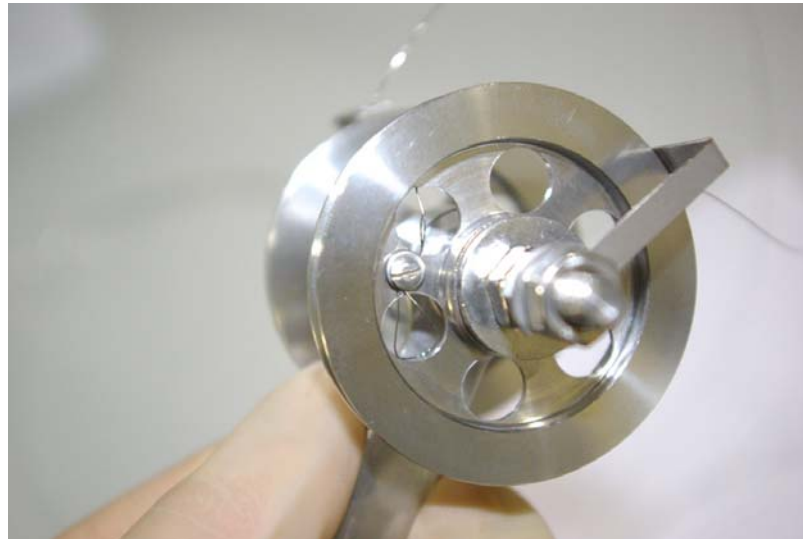
Figure 4 knot on the terminal of wire joining it to pulley by screw.
