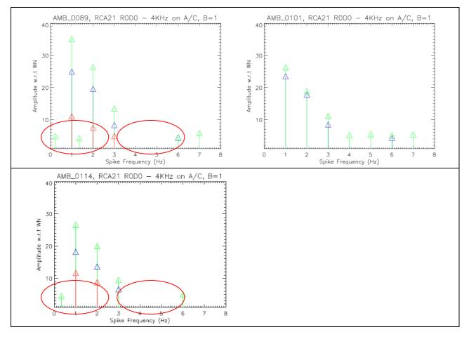
During the last System level tests not only the 1 Hz spike, and its harmonics, was visible but also some lower frequency spikes appeared. These spikes were totally unexpected and they were not visible in any of the WFTs performed during the QM/FM test campaign.
