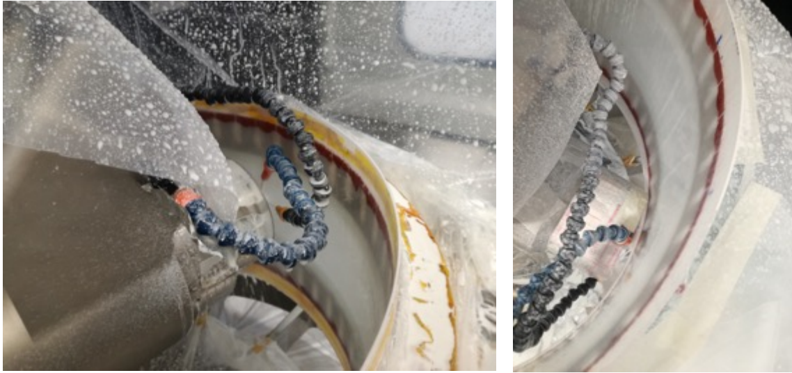
Figure 5: Configuration for polishing activity with Bonnet tool R20 on the shell#4. On the right, the set-up used on Parabolic side, on the left the protective system implemented on Hyperbolic side to prevent slurry sputtering outside the shell.
