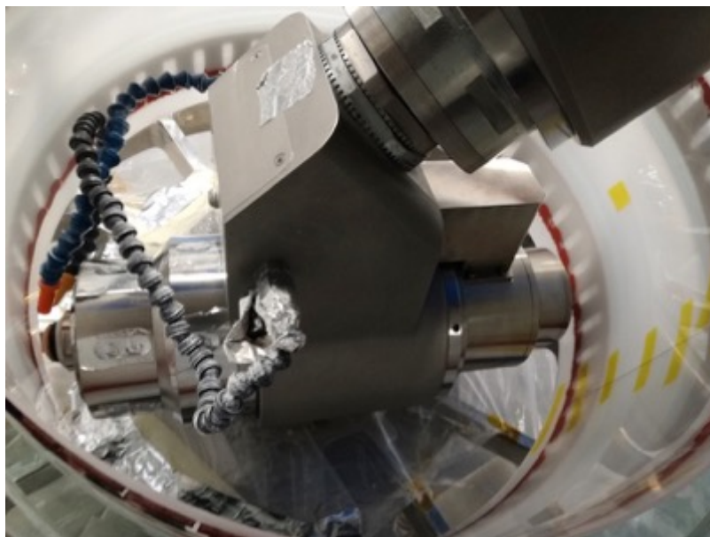
Figure 4: The Zeeko IRP1200 equipped with the Bonnet R20 is used @INAF/OAB to polish an azimuthal segment of the shell#4. Given the relative size of the shell and of the robotic arm, the accommodation of the shell was not simple. The precession angle is reduced to 10° and set in horizontal direction. In this way the shell fits with few millimeters margin. The breakage occurred on the lathe is visible on the right
