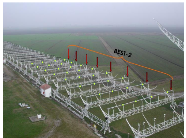
Fig. 4: The BEST-2 test bed is composed by 8 cylindrical concentrators with 4 receiver each.
