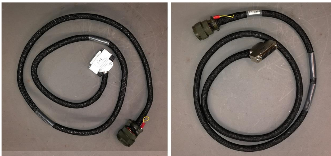
Figure 14 - Clock and Video-Bias cables (option 1)
