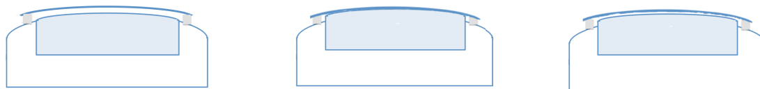
Fig. 9.: Sketch of the mould and glass foil inside the muffle. The gray spacers represent the sealing material we use to enable the pressure application. From left: the mould is at 0 level with respect to the muffle (PoC#2). The mould is in contact at room temperature with the glass foil (PoC#3). The mould is at an intermediate position defined with FEA (PoC#4)
