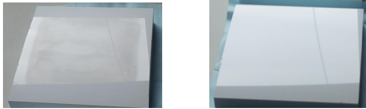
Fig. 3. Visual comparison of the surface roughness of the MK20-10 and MK20-20 (size 250 mm x 250 mm). Left) the MK20-10 shows the optical part (200mm x 200mm) with lower reflectivity due to a damaged surface. Patterns are also visible on the surface. Right) the MK20-20 with the homogeneous highly reflective surface.
