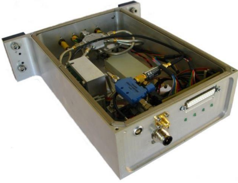
Fig. 16. Warm IF amplification module with integrated switch and digital attenuator.
