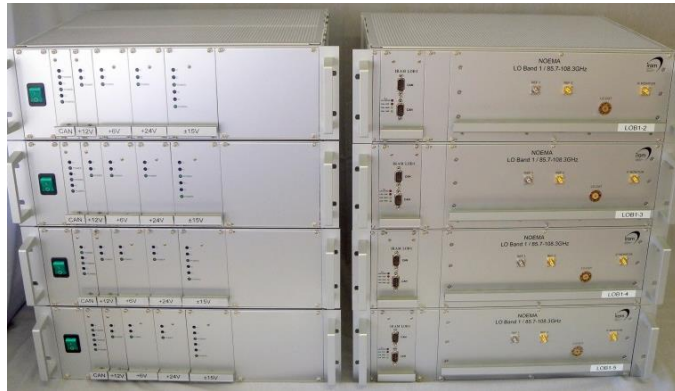
Fig. 13. The four production series of NOEMA Band 1 (~82-108.2 GHz) LO racks (right) and their power supply racks (left).
