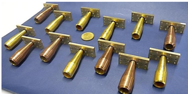
Fig. 8. Photo of some of the NOEMA Band 2 corrugated feed-horns.
