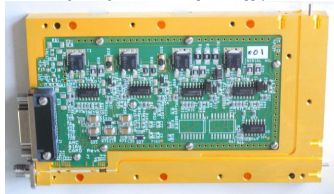
Fig. 11. Active Multiplier Chain developed for the NOEMA LO Band 1 system (AMC1) delivering a tuneable signal across \sim 82 -108.3 GHz and a power level of order \sim 12 dBm at its WR10 waveguide output.
