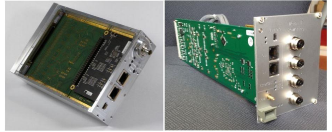
Fig. 18. EtherCat modules for biasing the NOEMA SIS junctions (left) and controlling the warm IF chain and laser rack emitter (right).
