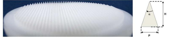
Fig. 4. Photo of HDPE vacuum window showing the triangular grooves on one of the surfaces (left). Geometry of the corrugations (right).
