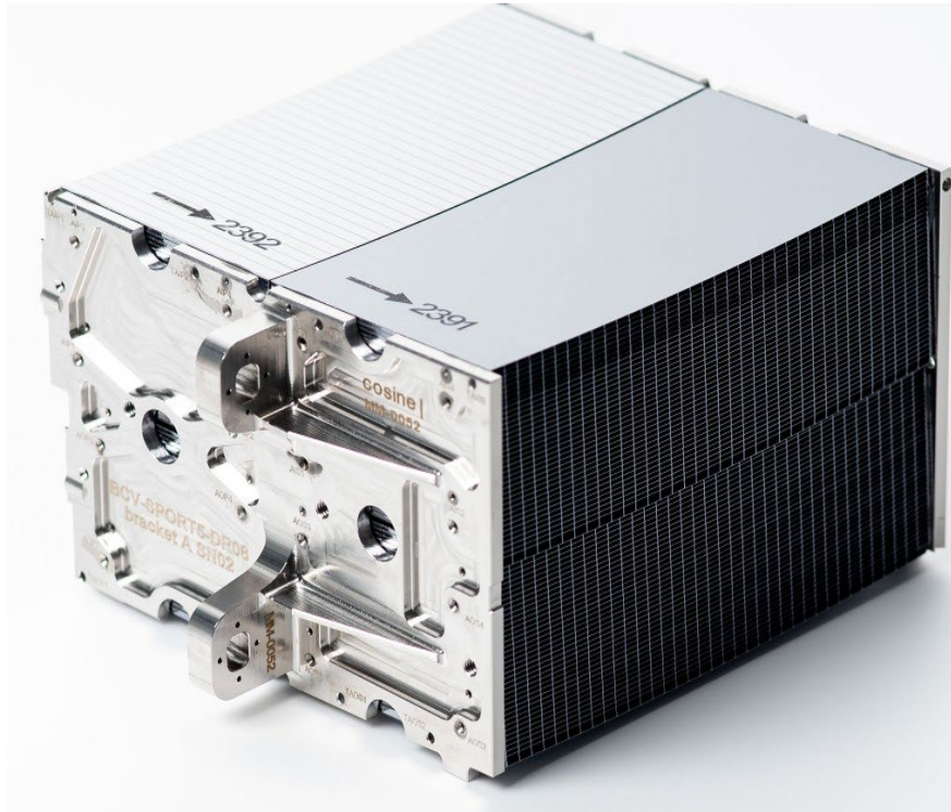
Figure 5: The NewATHENA optics consists of 492 SPO mirror modules, concentrically arranged in 13 rows; the figure shows a mirror module for the eighth row. The production processes used in the current development phase are largely the same as will be used for the flight implementation phase, ensuring a smooth transition between the phases. The actual mirror plates are only paper thin, 150 \mu\text{m} , and are fabricated with automated equipment spun in from the semiconductor industry, starting with 300 mm diameter, 0.775 mm thick latest generation Silicon wafers. Each mirror module consists of four stacks of mirror plates, carefully aligned using synchrotron radiation to produce a single focus. The four stacking robots required to produce the mirror stacks for the flight implementation phase (about 2500 including spares etc) already exist.
