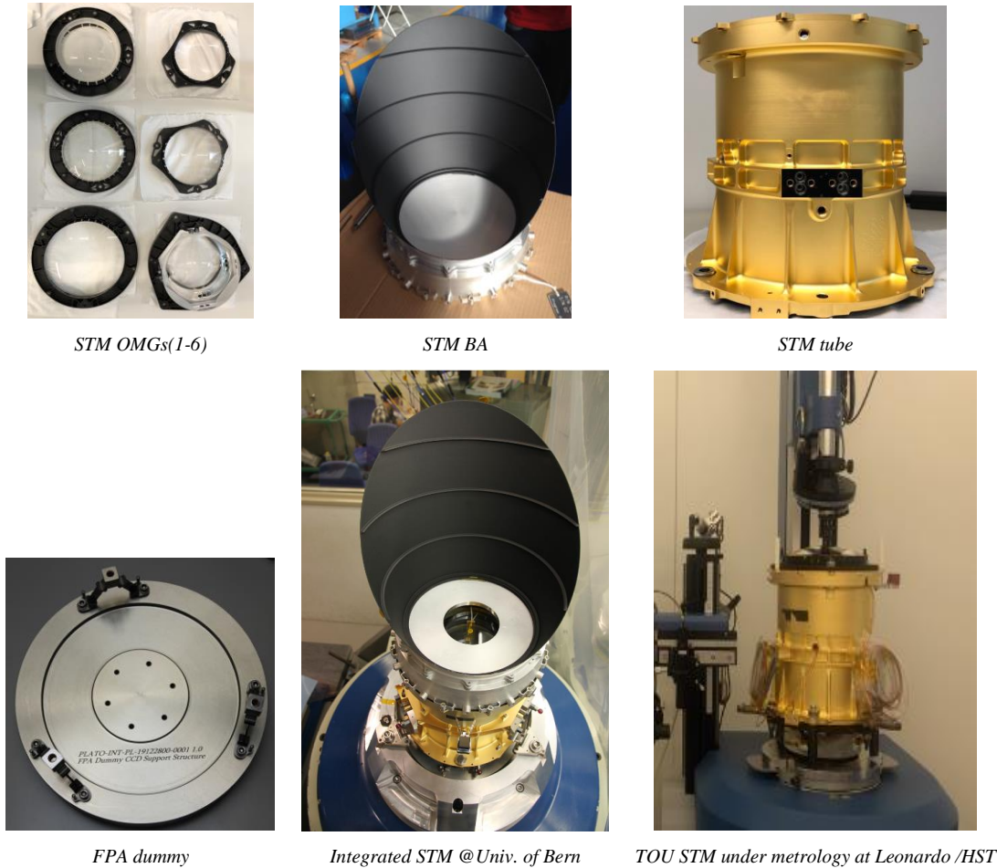
Figure 3 - TOU STM integrated, tested and successfully qualified at University of Bern. STM OMGs assembled and qualified by Leonardo; Baffle Assembly designed, manufactured and tested by Thales Alenia Space, Italy and Leonardo. FPA dummy provided by INTA.
