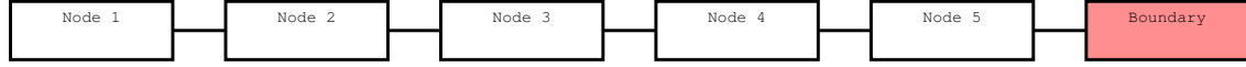
Figure 1: The numerical model used in the simulations. The temperature of the boundary node is specified by an analytical function or by a tabulated set of temperatures, depending on the test. We compare this boundary temperature with the temperature at node #1, at the other side of the bar.
