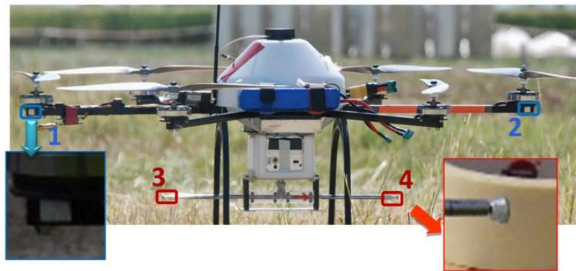
Fig. 6. Points used to estimate the relative orientation between the UAV direction and the transmitter antenna
