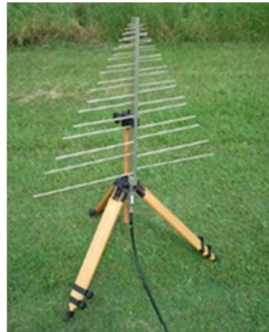
Fig. 8. The log-periodic antenna PMM LP-02
