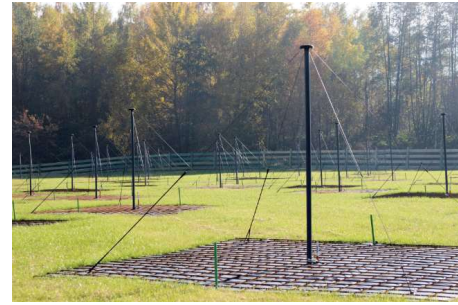
Fig. 1. Picture of the Low Band Antenna of LOFAR.
