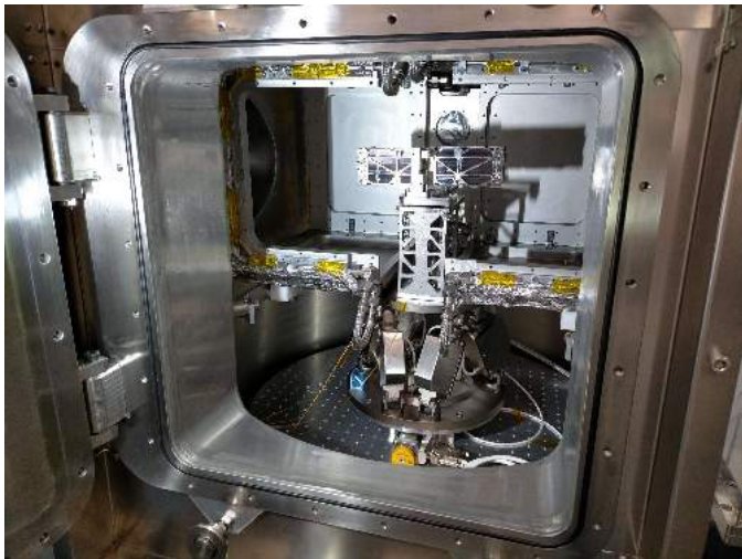
Fig. 4. SPO MM (MM-0042) installed inside the vacuum chamber on the support, which is also used for the Hartmann plate. The support is mounted on the hexapod for alignment in the expanded beam.
