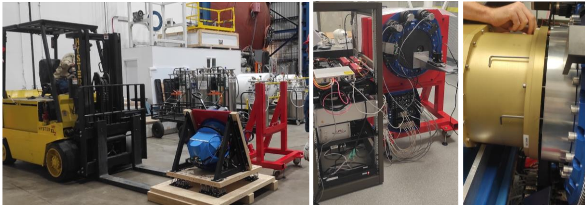
Figure 6: Pictures of Pre-Com-1 activities. Left : Optical bench removal from Box #1 and installation onto its handling. Center : SHARK-NIR instrument cabled inside LBT clean tent. A temporary lab camera was used in place of the scientific camera. Right : Scientific camera installation after its correct focus position has been determined.
