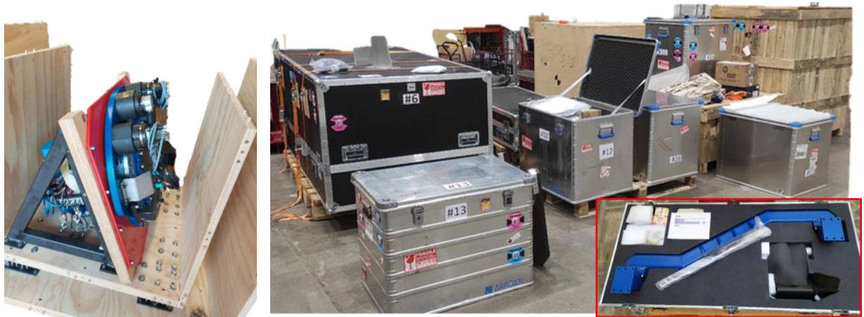
Figure 5: Left : Custom double-box with dumping system to ship the aligned optical bench (Box #1). Right : boxes after arrival at LBT premises. Tilt and shock sensors are visible. Red square . Custom box with pre-cut foam to transport the deployable arm (Box #3).
