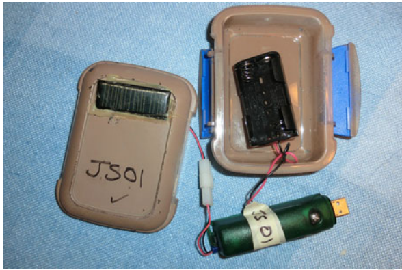
Fig. 8 Pressure and solar-flux logger used by Lorenz and Jackson (2015) and elsewhere. The commercial logger itself is essentially a USB memory stick ( green cylindrical object at lower right ) which can accommodate a single AA battery to operate for several days. Here a 2 \times AA battery holder (which due to peculiarities of the power supply system yields about a month of operation at 2 Hz) is included, as well as a solar cell to record the shadow of dust devils. The whole unit can fit in a pocket. Note the logger identifier, necessary as these loggers have been installed in arrays
