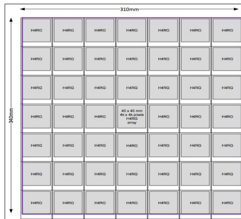
Figure 7. Top left : photograph of a Teledyne HR4G-10 HyViSI detector. Bottom left: schematical display of the focal plane with its 7 × 7 Teledyne detectors. Right: Characteristics of the Teledyne H4RG10-HyViSI detector.
