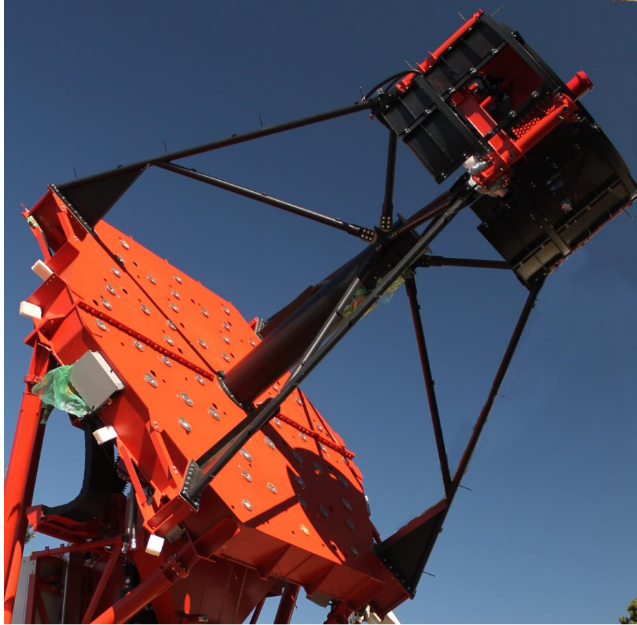
Figure 4: The optical supporting structure of the ASTRI SST-2M during its assembly at the telescope site. In the image the M1 dish, the mast and central tube, the M2 backup structure with the baffles.
