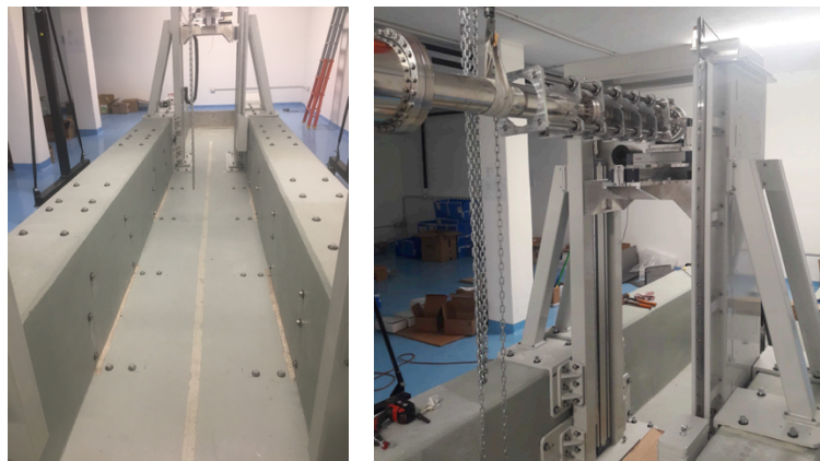
Figure 4: The detector tower. Left: holes to anchor the tower are prepared at f = 12 - 10 - 8 m, for flexibility of the facility. Right: The tower with the bellow for the focus search.
