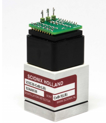
Figure 6: The assembly of the \text{CeBr}_3(\text{LB}) crystal and R11265U-200 with the 10X divider.
