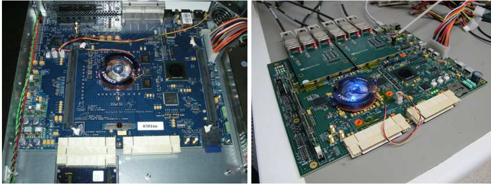
Fig. 1. ROACH1 (left) and ROACH2 (right) CASPER processing boards.
