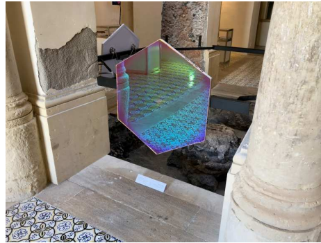
Fig. 4. The 85 cm hexagonal mirror of the Astri-Horn d'Arturo telescope at Serra La Nave
