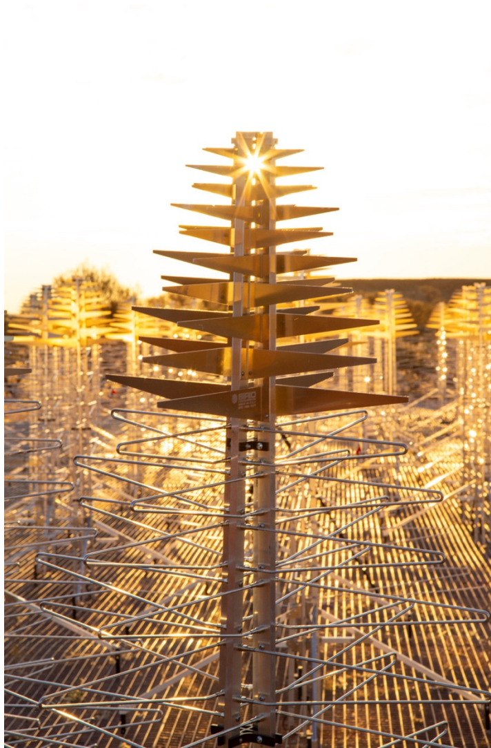
Figure 8. The SKALA (SKA Log-Periodic Antenna) 4.1 shown amidst a prototype station deployed at the Murchison Radio Astronomy site.
