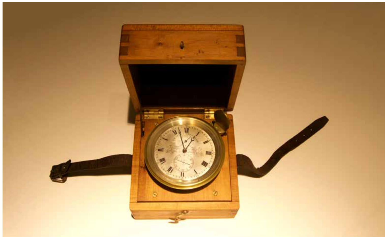
NA. 08. MARINE CHRONOMETER Charles Frodsham, London, second quarter of XIX secolo brass, silver and cherry wood INAF-Capodimonte Astronomical Observatory, Museum of Astronomical Instruments, inv. 1883
